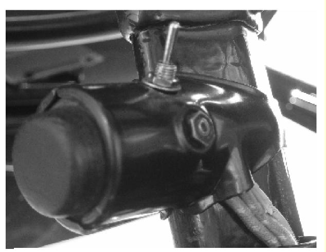
This shows the little switch mounted inside of the original horn button. It is quite a tight fit. For wires I used 22 gauge telephone wire.
