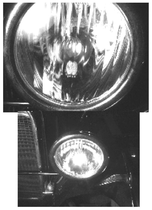
This shows the LED glued into the reflector. I mounted it so that it shines "up". This shows the front light "on".
