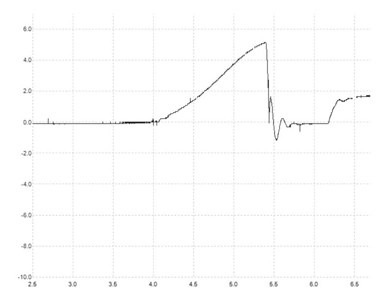
This graph corresponds to the timer closing at "point 6" on the voltage graph above. The timer has been advanced 22.5 degrees and closes at 3.6 ms, which is near the null point of the voltage waveform. The amperage builds to about 6 amps, which fires the coil at 5.4ms. This is the same situation as the first graph in this series, except the voltage is reversed.
