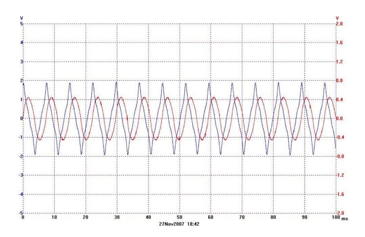
The voltage is now about 20 peak volts. The current, however is still at about four amps. The current essentially stays the same because as a load, the model T coil is mostly reactive. This means that as the magneto tries to put current into the T coil, the T coil tries to put current back into the mag. The faster the mag tries to put the current in, the more the coil resists and a sort of equilibrium is reached.
