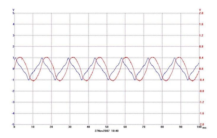
The speed of the magneto was 500 rpm. The voltage is the spiky waveform and the current is the smooth waveform. The voltage is about ten peak volts and the current is about four amps. Most ac voltmeters show rms voltage. Rms voltage is equal to the dc voltage value that would produce the same amount of heat as the ac voltage. For the model T magneto waveform the rms voltage is about 1/2 of the peak voltage.
