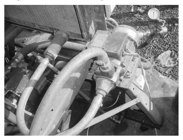
For water and oil circulation I used impeller pumps. I plumbed the water lines with half inch flexible hose. The radiator is an old car radiator cooled with a box fan.
