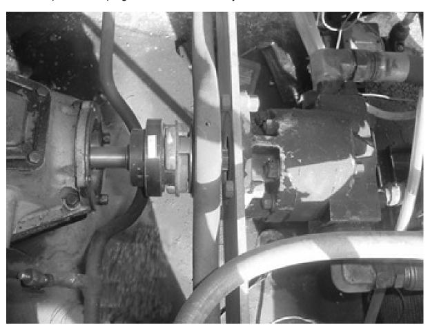
This is a shot of the T motor coupled to the pump. The coupler has a piece of reflective tape for use with the optical tachometer.
