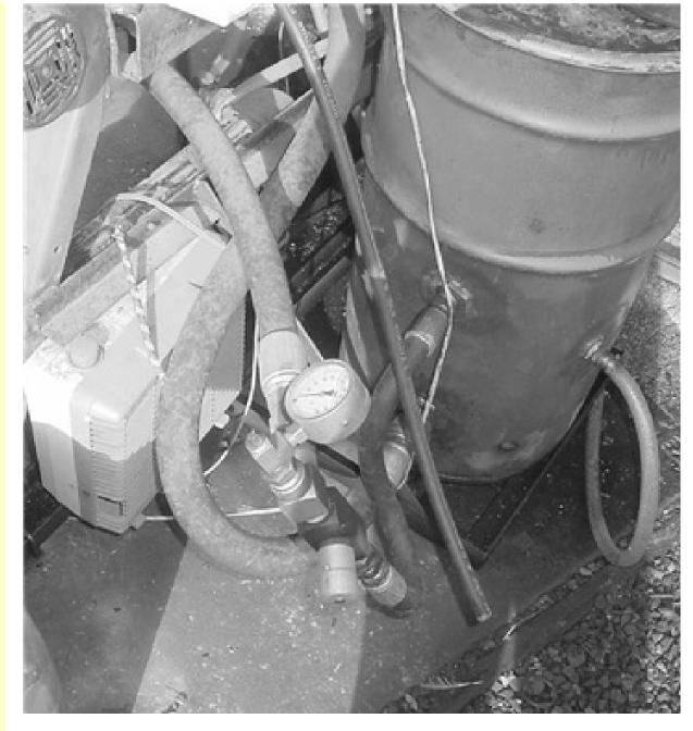
This shows the oil storage tank, the restrictor valve and the oil cooling fan. I ran the oil through a small radiator to help cool it too.
