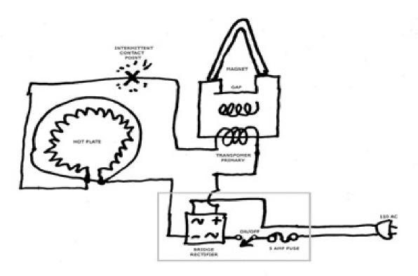
The "X" on the schematic denotes a break point in the circuit where the DC to the transformer is made and broken. To charge a magnet does not require a steady shot of
