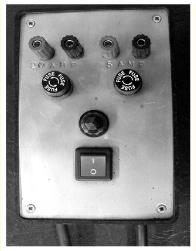
5 amp fuse and holder. Switch, Power, cord Hot plate.
