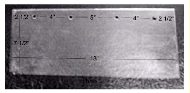
Use some modeling clay to fill the sparkplug hole flush. Invert the head and stabilize it so that the valve side is slightly lower. Place the Plexiglas onto the deck, sealing it with the grease. Proceed to fill the chambers with water from the syringe, being careful to keep track of how much water you use.
