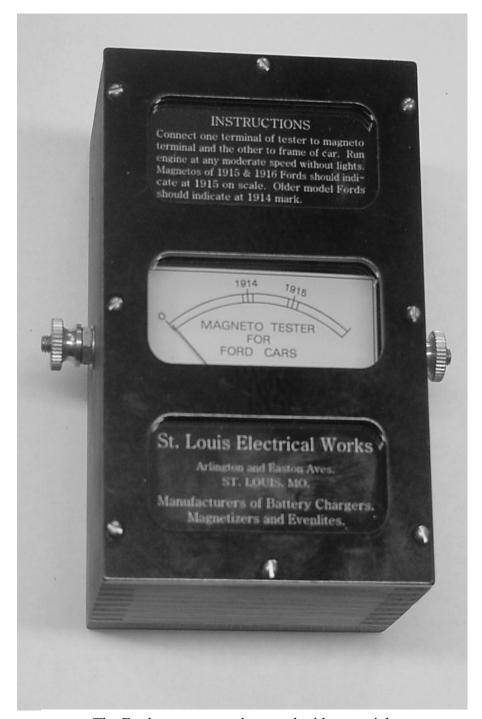
The Ford magneto can be tested with a special magneto tester. This instrument is nothing more than an ammeter, but one provided with a "reactance coil" which enables the meter to indicate a constant current at all speeds. In other words, the meter is so designed that it will indicate if the magneto is giving its proper output at any speed of the engine, while testing.
