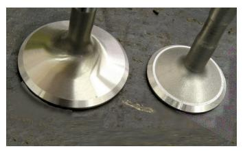
Swirl polished valve on left, regular valve on right. This is done ostensibly to increase the flow characteristics of the valve. I think the results are dubious at best and short lived, as the valves carbon up in a few miles, obliterating the swirl finish.
